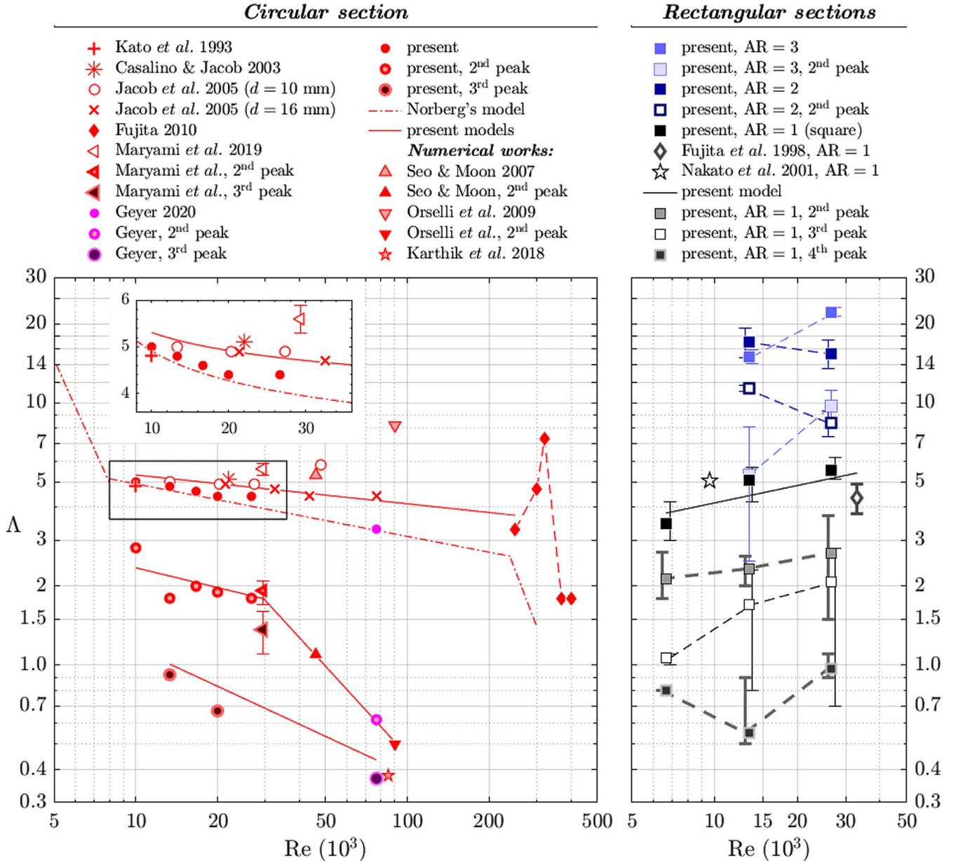
**Fig. 11.** Spanwise coherence length according to definition (2) in flows around circular and rectangular cylinders, at first (left) peak unless otherwise stated. Uncertainty bars cover several probe locations. If so, the symbol is at the mean. Dashed lines for visual aid only.
