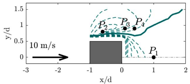
**Fig. A.1.** Mean flow over a rectangular cylinder of  $AR = 1$  (square cylinder)  $Re = 6,700$ . Isocontours of velocity norm from  $0.4 U_\infty$  to  $1.6 U_\infty$  by step of  $0.1 U_\infty$ . The full, thick line is where  $U = U_\infty$ . The labeled bullets ( $\bullet$ ) are the position of the probes in the spanwise study.
