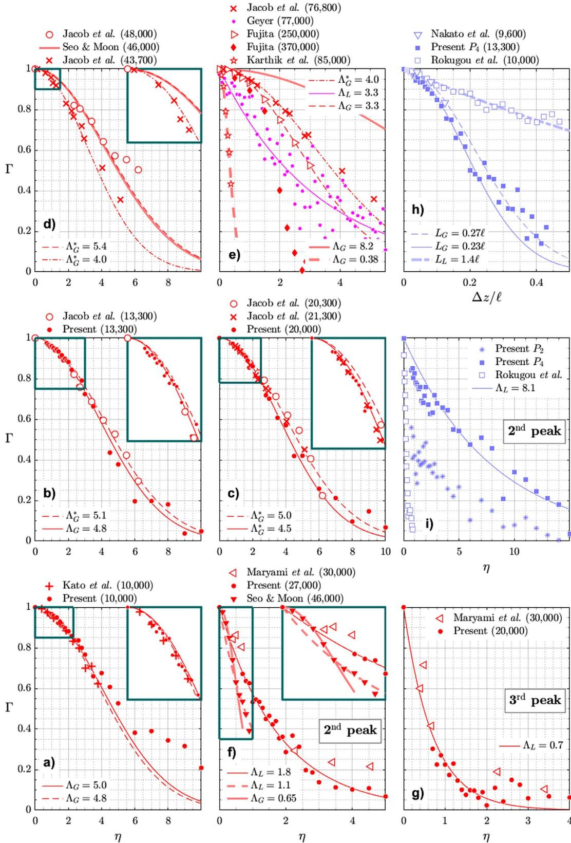
**Fig. B.2.** Spanwise coherence data (symbols) and model (lines) for the flow over a circular (a–g) and a rectangular of AR = 3 cylinder (h, i). Literature data and models have been obtained as described in Appendix B. Data from Maryami *et al.* [14] are for  $\theta = 135^\circ$ . In (e), the line  $\Lambda_G = 8.2$  accounts for the numerical data reported by Orselli *et al.* [25] (Re = 90,000). The Reynolds numbers in (i) are the same as in (h).
