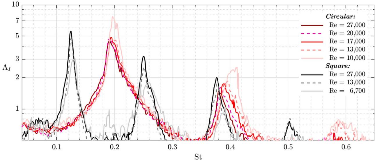
**Fig. 8.** Frequency dependent, normalized spanwise coherence length in the flow over circular and square cylinders, estimated from integration of coherence data (3). Measurements at  $P_4$  for the square section. Results at other probe locations are available in the [Supplementary file](#).
