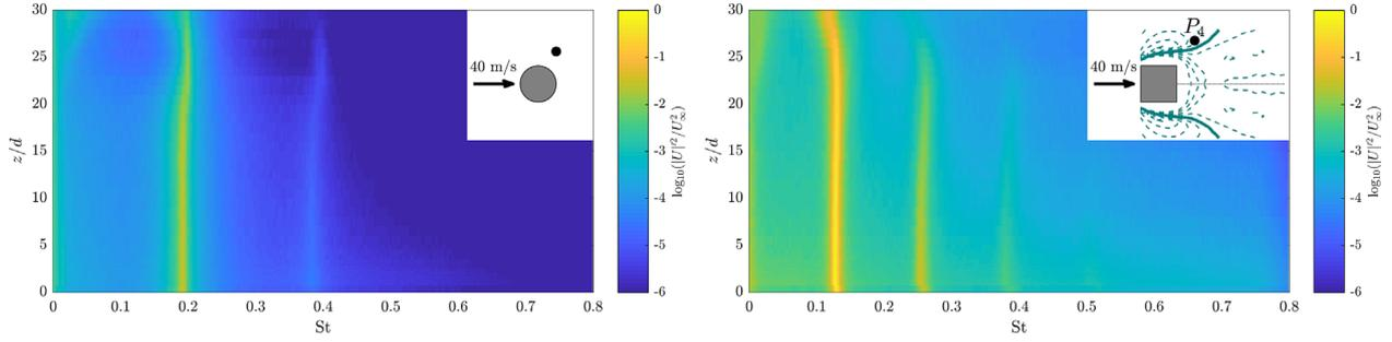
**Fig. 3.** Spanwise distribution of the velocity power spectral density for the flow over the circular (left) and square (right) cylinders, at  $Re = 27,000$ . Inset is the case. The black bullet ( $\bullet$ ) indicates the probe position and the lines are mean flow velocity contours (see Sect. 2.3.1).
