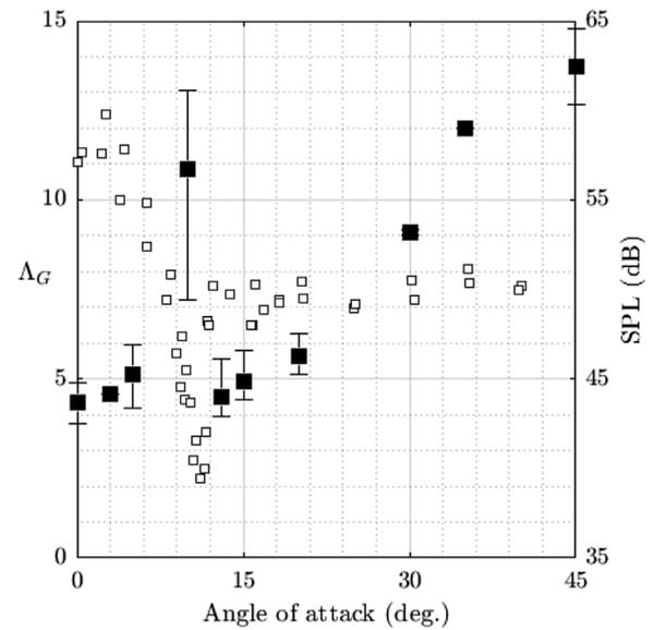
**Fig. B.1.** Coherence length (■ with error bars) and Sound Pressure Level (SPL, □) for a 20 mm side square cylinder at incidence in a flow at 25 m/s, according to Fujita *et al.* [23]. Note that the coherence length is given as normalized by the square side, which does not correspond with the body height at incidence (referred to as “the effective geometrical width normal to the flow” by the Authors).
