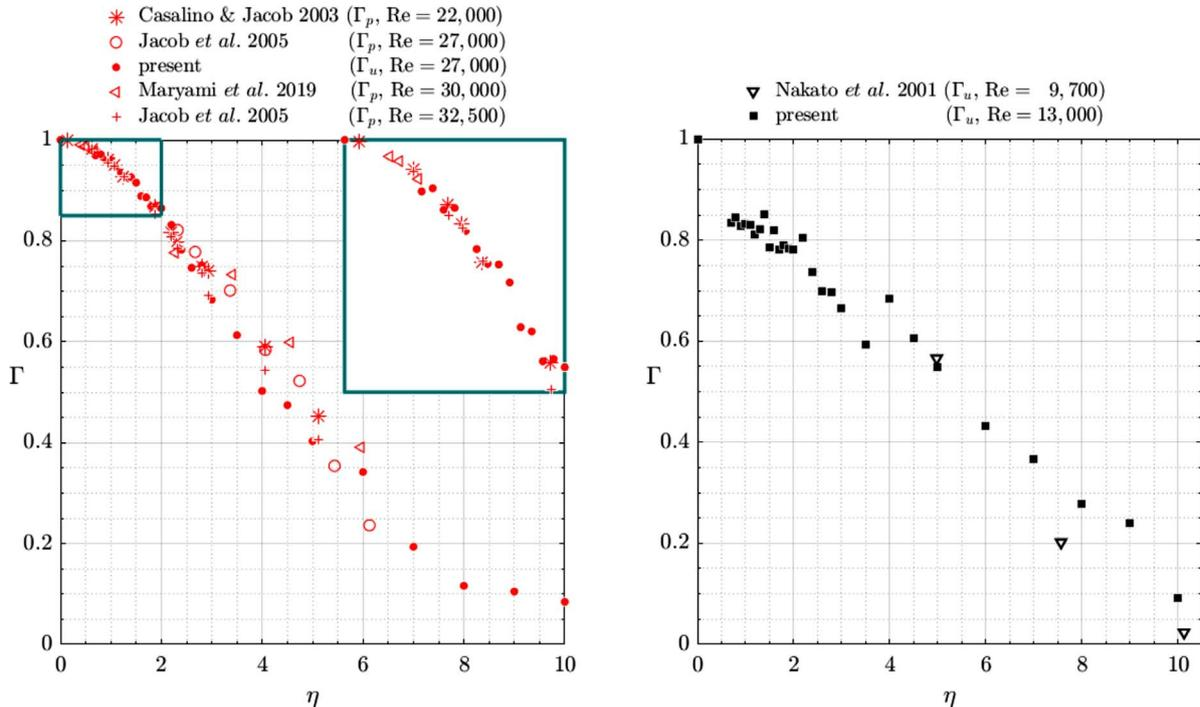
**Fig. 4.** Spanwise coherence data in the flow over the circular (left, probe at  $(x, y) = (0, 0.9d)$  for present data) and square (right, probe at  $(x, y) = (1.0d, 0)$  for both data-sets) cylinders, at the main peak frequency ( $St = 0.193$  and  $0.125$  for present data on left and right, respectively).
