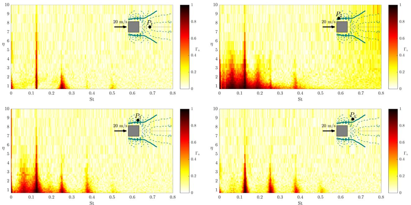
**Fig. 6.** Spanwise coherence of the velocity ( $\Gamma_w$ ) in the flow over the square cylinder, at Re = 13,000. Inset, the black bullet (•) indicates the probe position and the lines are mean flow velocity contours (with same legend as Fig. 5).
