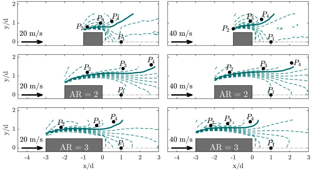
**Fig. 5.** Mean flow over a rectangular cylinder of AR = 1 (square cylinder, top), 2 (middle) and 3 (bottom) at Re = 13,000 (left) and Re = 27,000 (right). Isocontours of velocity norm from  $0.4 U_\infty$  to  $1.6 U_\infty$  by step of  $0.1 U_\infty$ . The full, thick line is where  $U = U_\infty$ . The labelled bullets (•) are the position of the probes in the spanwise study. The case AR = 1,  $U_\infty = 10$  m/s is shown in Figure A.1.
