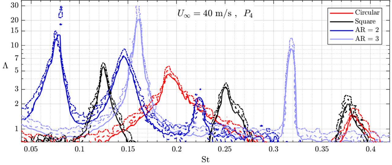
**Fig. 7.** Frequency dependent, normalized spanwise coherence length in the flow over cylinders, at  $Re = 27,000$ . Measurements at  $P_4$  for rectangles (see Sect. 2.3.1). Full lines: estimation from spanwise integration of coherence data (3); dashed and dash-dotted lines show isocontours of  $\Gamma_u = \exp(-\pi/4)$  and  $\Gamma_u = \exp(-1)$ , respectively, in the  $(\eta, St)$  field, corresponding to a coherence decay assumed as either Gaussian or Laplacian, respectively.
